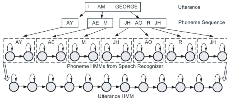
Figure 3.4: The utterance transcription is parse into the correspondent sequence of phonemes. The HMMs for each phoneme is retrieved from the speech recognizer and concatenated to form a single utterance HMM.
