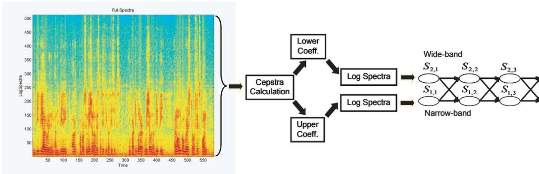
Figure 5.2: Multiband model for the wide/narrow band partition.
