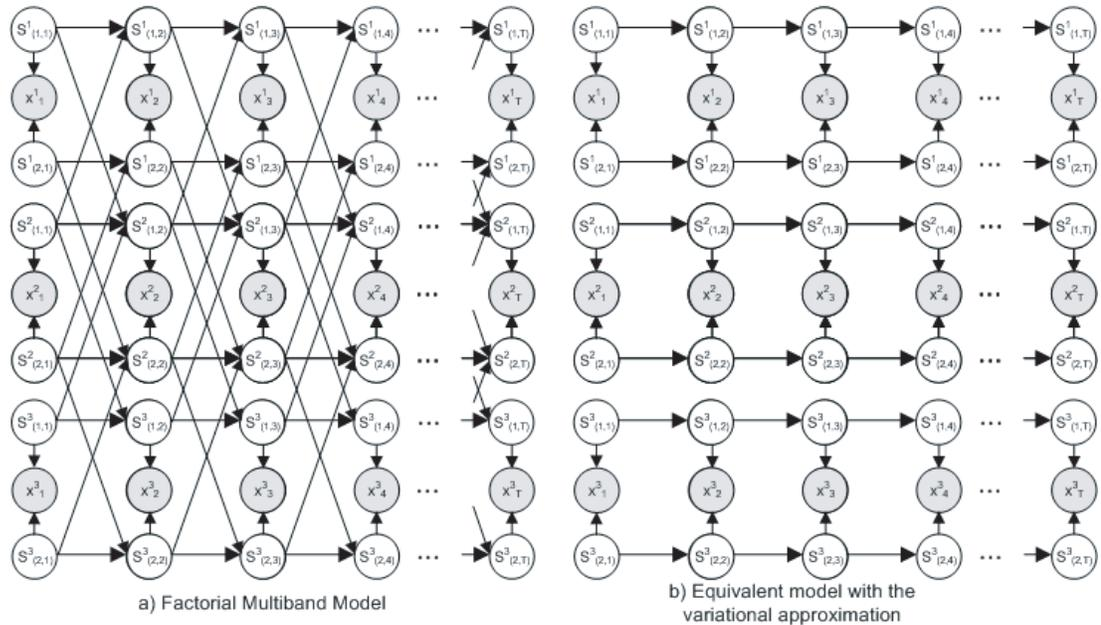
Figure 5.3: a) Factorial Multiband Model b) The proposed variational approximation decouples the factorial HMMs (FHMM) into individual FHMMs per band.
