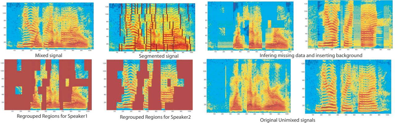
Figure 7.4: The first row shows the original mixed signal. Second row shows the re-grouped signals by the spectral clustering algorithm. The third rows shows the reconstructions of the “missing” regions. Fourth row shows the original signals prior to the mixing.
