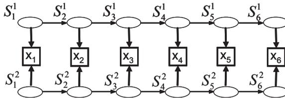
Figure 3.5: Factorial HMM for two speakers (two chains).
