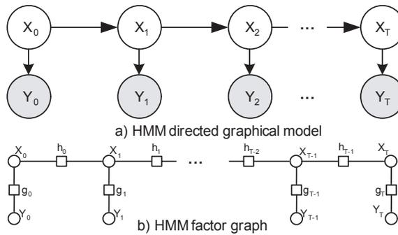
Figure 2.1: a) An HMM as a directed graphical model, b) HMM factor graph representation, where  $g_t = p(Y_t | X_t)$  and  $h_t = p(X_{t+1} | X_t)$
