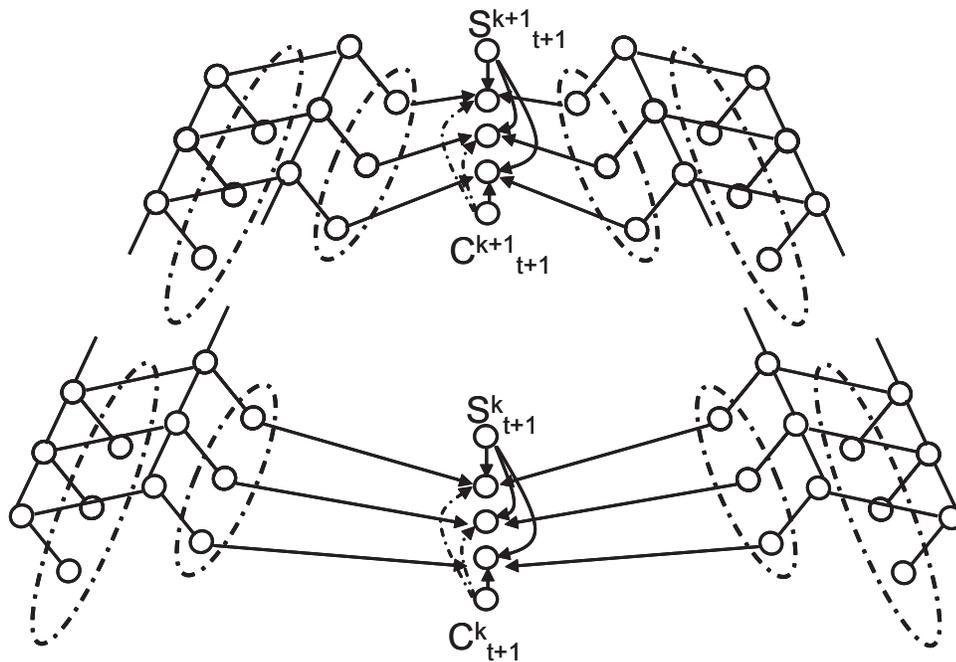
Figure 7.2: Subband version of the match-and-track model. Each subband  $r$  with  $\mathcal{K}_r$  spectral coefficients has its own state,  $S_t^r$ , and switching,  $C_t^r$ , variables
