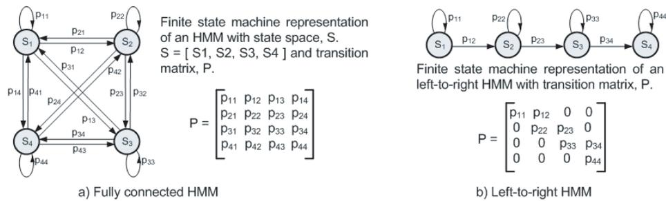
Figure 1.3: a) Finite machine state representation of a fully connected HMM. b) Finite machine state representation of a left-to-right HMM.
