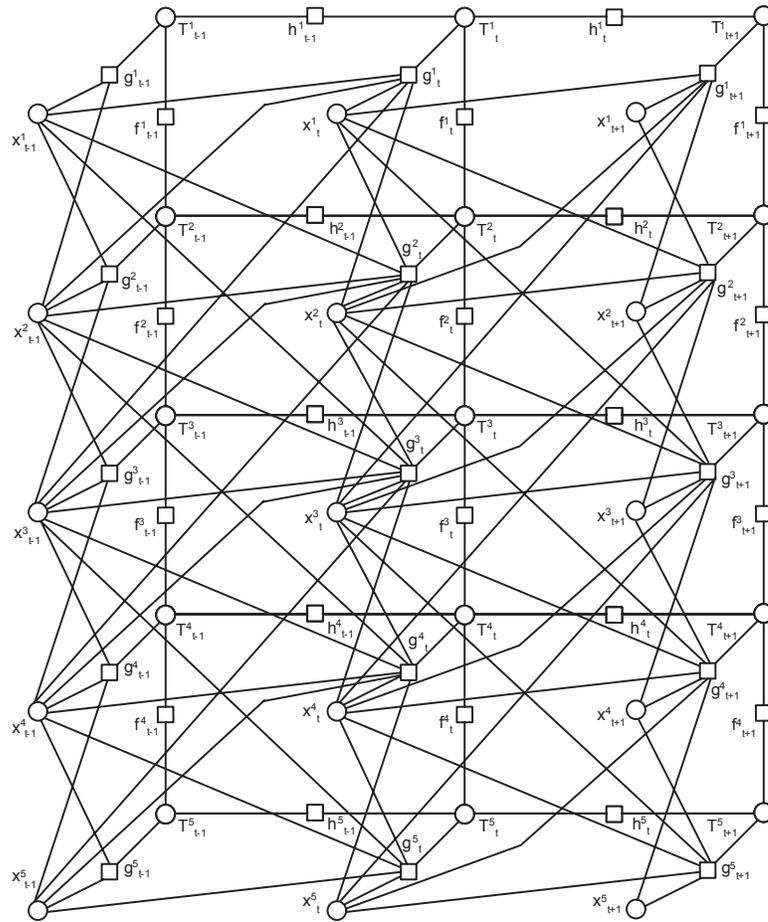
Figure 6.4: Factor Graph for the relationships between spectrogram bins  $x_t^k$  and transformation nodes  $T_t^k$ . Function nodes  $g_t^k$  correspond to the “local-likelihood” potentials (eq. 6.6). Function nodes  $h_t^k$  and  $f_t^k$  correspond to the horizontal and vertical potentials.
