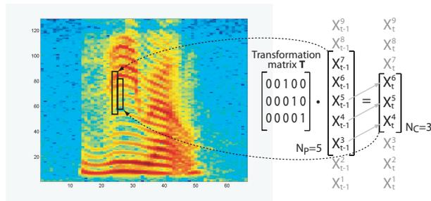
Figure 6.1: The  $N_C = 3$  patch of time-frequency bins outlined in the spectrogram can be seen as an “upward” version of the marked  $N_P = 5$  patch in the previous frame. This relationship can be described using the matrix shown.
