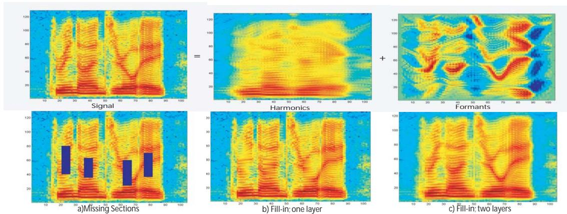
Figure 6.8: First Row: Harmonics/Formants decomposition (posterior distribution means). Second Row: (a) Spectrogram with deleted (missing) regions. (b) Filling in using a single-layer transformation model. (c) Results from the two-layer model.
