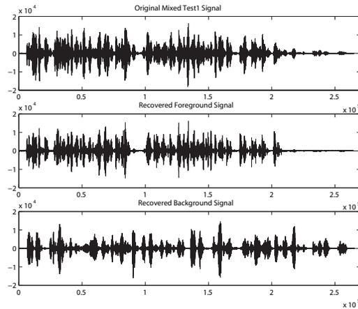
Figure 3.7: Input and output signals from complete system using factorial models and factorial processing.
