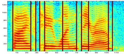
Figure 6.13: Frames selected by the matching-tracking model for a single source signal.
