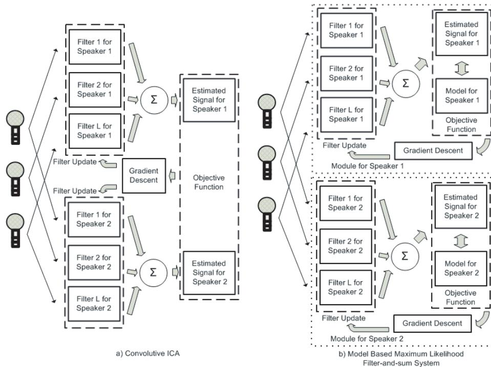
Figure 3.2: a) Filter Optimization for convolutive ICA; b) Proposed model-based optimization.
