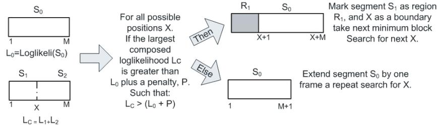
Figure 7.3: Schematic of the BIC segmentation procedure
