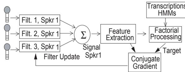
Figure 3.6: Complete system with speaker model produced by factorial processing.
