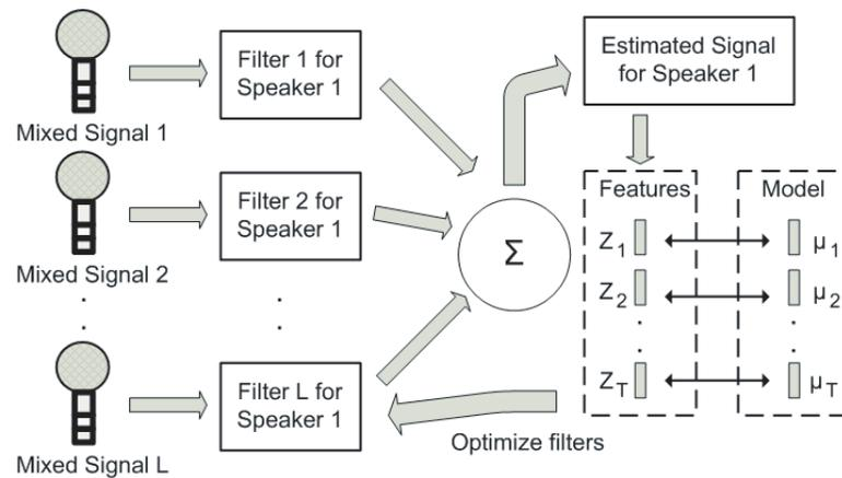
Figure 3.3: The goal is to optimize the filters such that the features derived from the estimated speaker at frame  $t$ ,  $z_t$  resembles the features described by the model,  $\mu_t$
