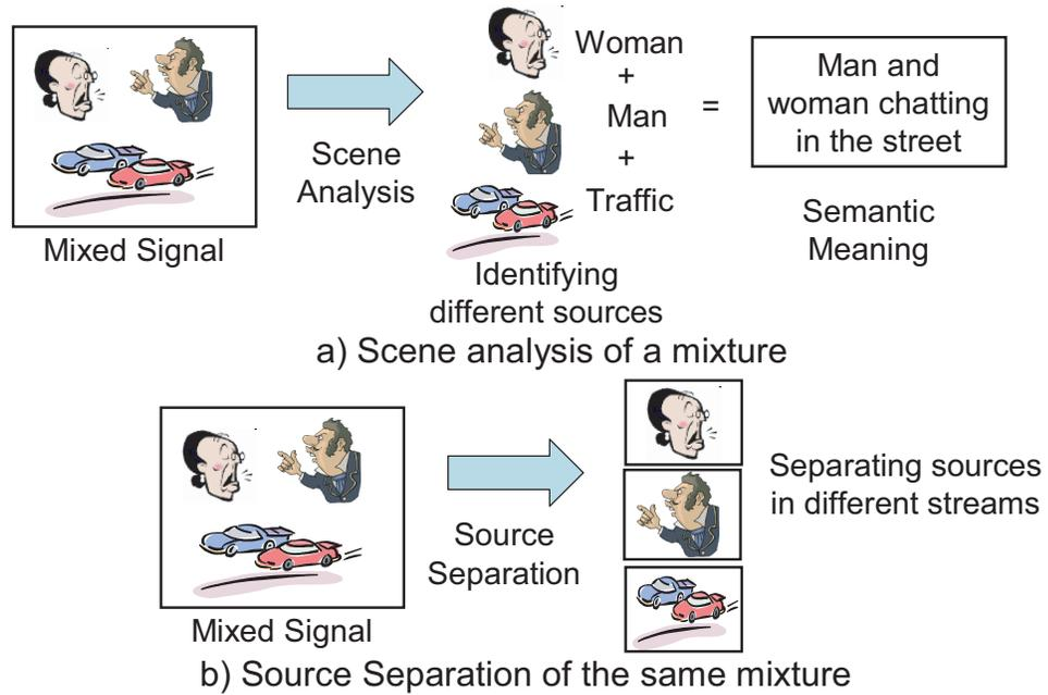
Figure 1.1: a) Scene analysis and b) source separation of the same mixed signal.
