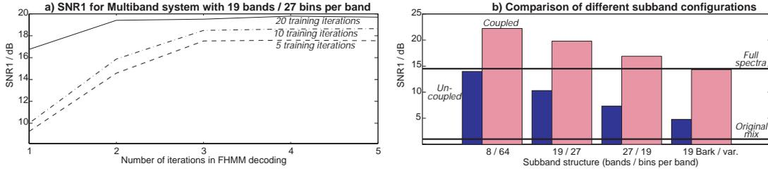
Figure 5.4: a) SNR1 for a 19-band system versus iterations in recognition and training. b) SNR1 for different structures of independent and coupled multiband systems, where the first bar in each pair corresponds to the independent model and the second to the proposed coupled model.
