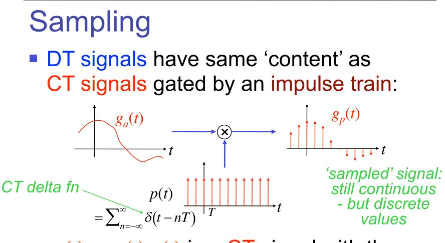
g<sub>p</sub>(t) = g<sub>a</sub>(t)·p(t) is a CT signal with the same information as DT sequence g[n]
