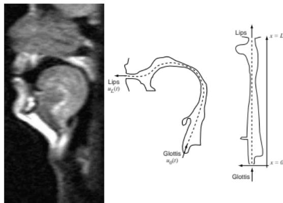
Discrete approximation as varying-diameter tube
