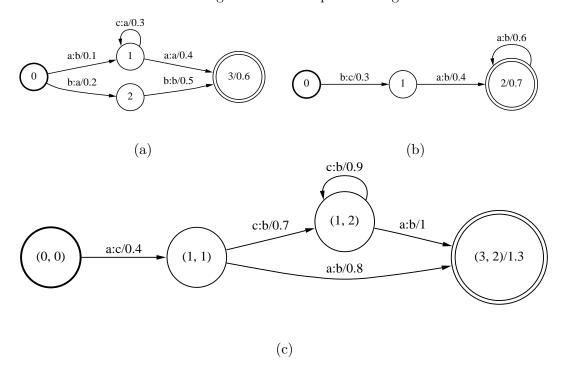
**Figure 3:** Example of transducer composition.
