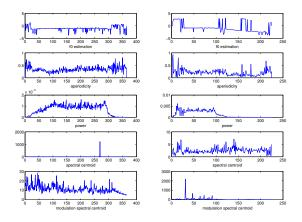
Figure 2: Features extracted from a blender sound at left, with the human imitation at right. Five perceptual features:  $f_0$  estimation, residual (aperiodicity), power estimation, spectral centroid and modulation spectral centroid. Time segemnts on the horizontal axis, feature output on the vertical axis.
