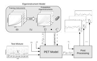
**Figure 1**. Illustration of the *Probabilistic Eigeninstrument Transcription* (PET) system. First, a set of training instruments are used to derive the eigeninstruments. These are then used by the PET model to learn the probability distribution P(p,t|s), which is post-processed into sourcespecific binary transcriptions,  $T_1, T_2, \ldots, T_S$ .
