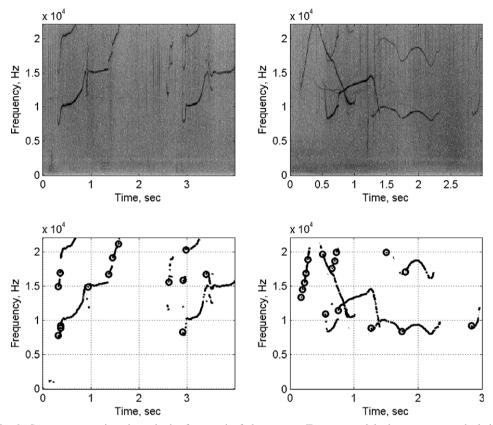
Fig. 3. Segment extraction through the front-end of the system. Top row: original spectrograms depicting multiple calls. Bottom row: extracted segments. Circles indicate sample segment edges for two different recordings.
