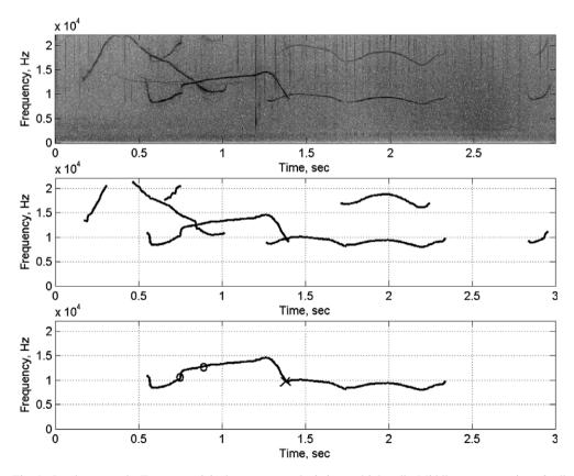
Fig. 6. Overlap example. Top row: original spectrogram depicting multiple calls. Middle row: extraction of calls. Bottom row: example calls. Circle indicates correct connection; × indicates false connection.
