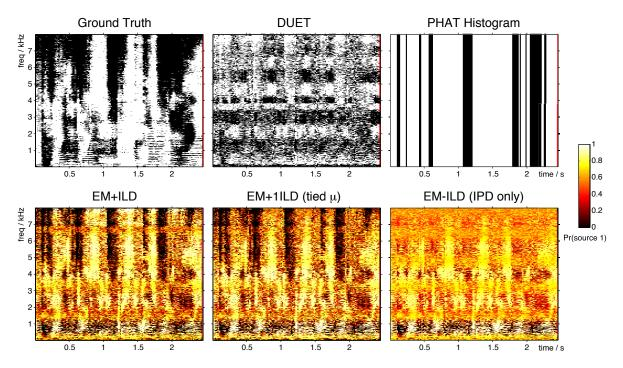
Figure 1: Example mask created by each algorithm for the same source in the same mixture of two sources separated by 75° in reverberation.
