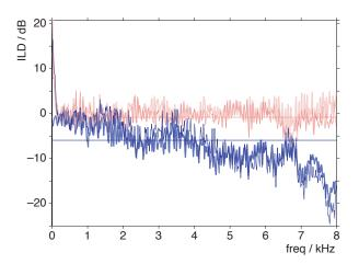
Figure 3: ILD as a function of frequency for two speakers separated by 75° in reverberation. The thin lines are our best ILD estimates for each source, the horizontal lines are ILD estimates when tied across frequency, and the thick lines are the ground truth ILDs. Light lines are speaker 1, dark for speaker 2.
