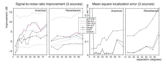
Figure 2: SNR improvement and MSE localization error comparison. "EM+ILD" is the full ILD/IPD based system; "EM+1LD" assumes that ILD is constant across frequency; "EM-ILD" is the IPD-only system; "Aarabi" is the approach from [2]; "DUET" is the approach from [5]; "gnd truth" is the optimal SNR from the oracle time-frequency mask; "random" uses a random mask.
