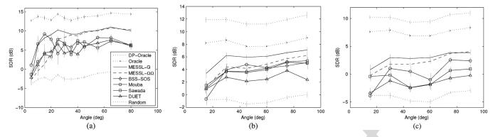
Fig. 7. SDR as a function of angle for three conditions. Anechoic conditions are averaged over ten mixtures at each of 12 angles, reverberant over 15 mixtures at each of six angles. Error bars show one standard error. (a) Anechoic, three speakers; (b) reverberant, two speakers; (c) reverberant, three speakers.
