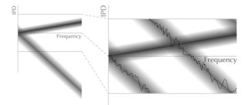
Fig. 1. Caricature of our probabilistic model of interaural phase difference (IPD) as a function of frequency, equation (5). On the left are the probability density functions (pdfs) of two competing model predictions, equation (3), where the IPDs are centered around their respective  $\omega \tau$  values. On the right, those pdfs are constrained to the interval  $(-\pi, \pi]$  so that the likelihood of the observation, equation (2), the dotted line, can be evaluated under each.
