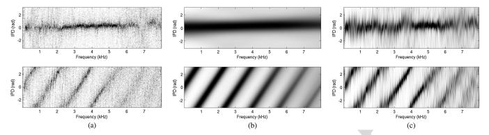
Fig. 4. Interaural phase differences (IPD) as a function of frequency for two speakers at  $0^{\circ}$  and  $75^{\circ}$  in reverberation. Black is higher probability. (a) Histogram of each source's IPD before mixing, (b) pdf of each source's IPD estimated from the mixture by MESSL using frequency-independent parameters,  $\Theta_{11}$ . (c) PDF of each source's IPD estimated from the mixture by MESSL using frequency-dependent parameters,  $\Theta_{\Omega\Omega}$ .
