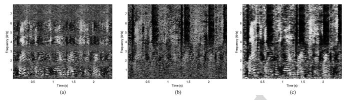
Fig. 2. Contribution of (a) IPD and (b) ILD to (c) MESSL mask using frequency-dependent  $\Theta_{\Omega\Omega}$  parameters. White is 1, black 0. Two speakers at  $0^{\circ}$  and  $75^{\circ}$  in reverberation. Notice that the IPD mask is mainly informative for low frequencies and the ILD mask for high frequencies, but not exclusively. For this same example, Figs. 3 and 4 show the ground truth and estimated parameters for interaural level and phase differences, respectively.
