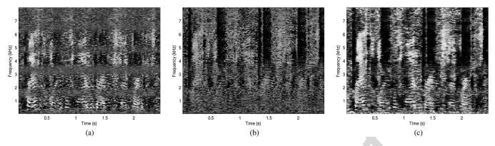
Fig. 2. Contribution of (a) IPD and (b) ILD to (c) MESSL mask using frequency-dependent  $\Theta_{\Omega\Omega}$  parameters. White is 1, black 0. Two speakers at  $0^{\circ}$  and  $75^{\circ}$  in reverberation. Notice that the IPD mask is mainly informative for low frequencies and the ILD mask for high frequencies, but not exclusively. For this same example, Figs. 3 and 4 show the ground truth and estimated parameters for interaural level and phase differences, respectively.
