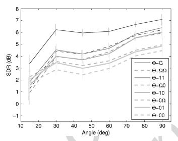
Fig. 6. Signal-to-distortion ratio for complexity experiment, two speakers in reverberation. Each point is the average of 15 mixtures with the same angular separation. Error bars show one standard error. Note that the random and DP-Oracle masks bound performance between 11.79 and -0.78-dB SDR, respectively, independent of angle.
