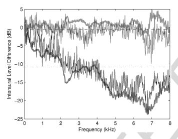
Fig. 3. Example ILD for two sources at  $0^\circ$  (upper lines) and  $75^\circ$  (lower lines) in reverberation. Thick lines are ground truth direct-path ILD measured in isolation, thin lines are estimated from a mixture by MESSL using frequency-dependent  $\Theta_G$  parameters, and the dashed lines are estimated by MESSL using frequency-independent  $\Theta_{11}$  parameters.
