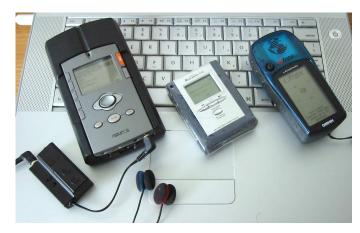
Figure 1. Data capture equipment. On the left is the Neuros hard-disk recorder, shown with the Soundman in-ear microphones and interface module. Middle is the mobiBLU flash-memory recorder. On the right is a logging personal GPS unit.
