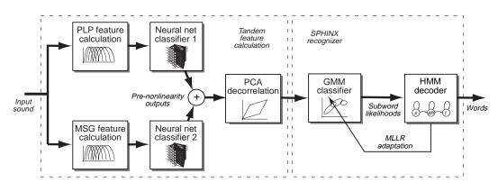
Fig. 1. Block diagram of the tandem recognizer used for the SPINE1 task.
